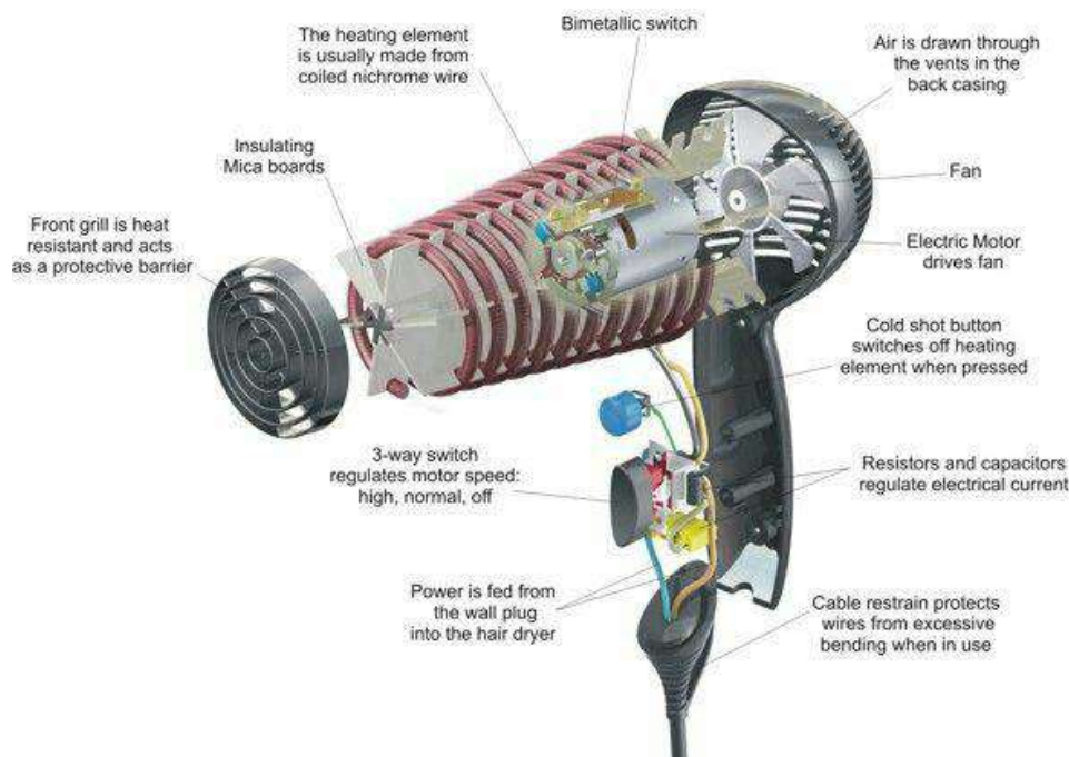
Fig 3.1 A hair dryer and its internal parts.
