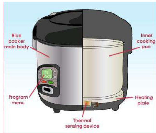
Fig 2.30 The inner workings of a typical rice cooker
