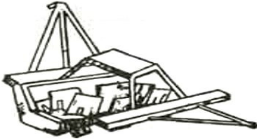
Figure: 3.7 Open blade puddler
