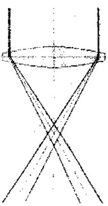
Fig 2.14 Chromatic aberration caused by a convex lens
