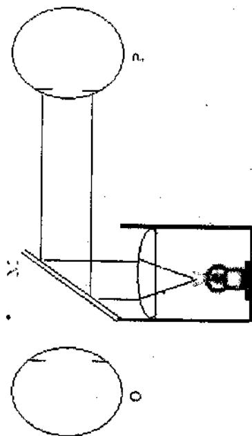
**Fig 12.2** Observation and illumination system in self illuminated retinoscope. 'O' stands for observer. 'P' stands for Patient. 'M' stands for Mirror
